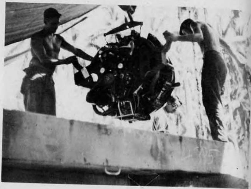
Above: Installing new motor in reconditioned LVT hull. Below: Salvaged tracks to be sent back to LVT repair base, Regular Navy outfit on Banika, for reconditioning.
