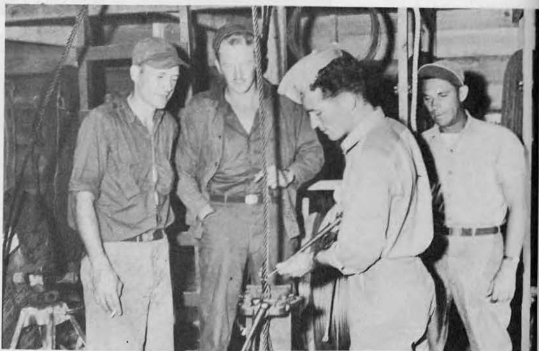
It takes riggers to keep supplies moving via heavy cranes. In the rigging loft, Chief John K. Baxter splices a steel cable. Looking on, left to right, are Lawrence Elmore, Paul F. Barker and Harry R. Gregory, all boatswains mates.
