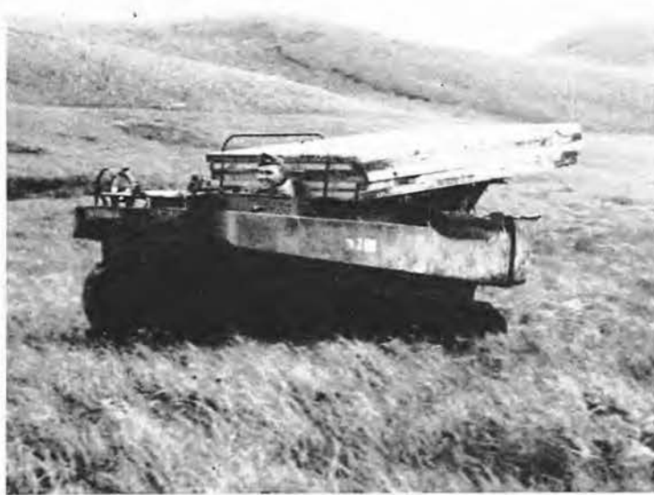
THE TUNDRA TIGER—as we called this swamp buggy or snow jeep—hauled some of the camp-building material from the beach to the site.
