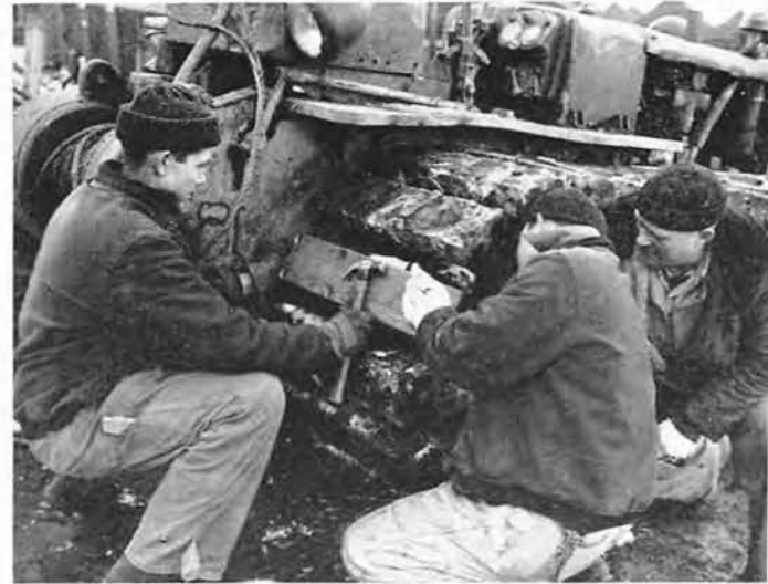
PUTTING SNOWSHOES on a “cat” was just one of the more unusual jobs we were called upon to perform. Wooden cleats added to traction sur-
