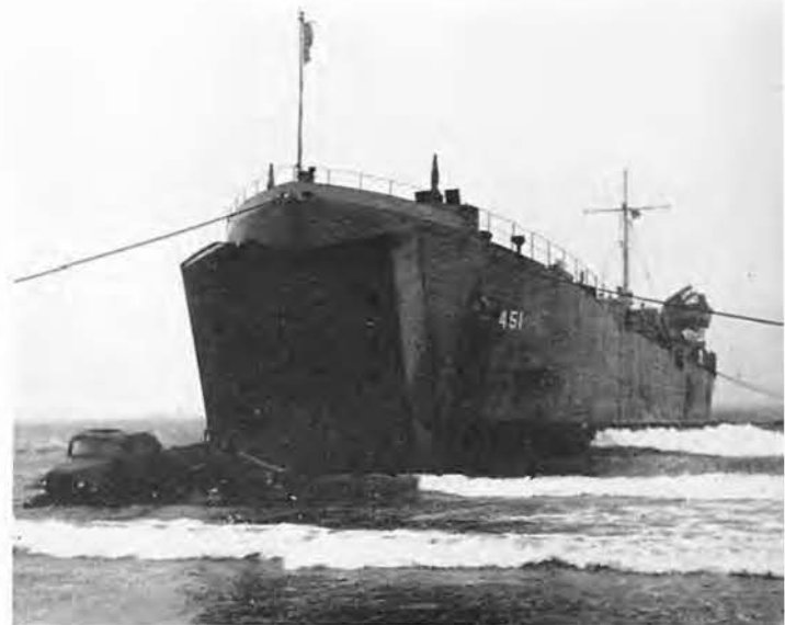
WE UNLOADED CARGO through the churning surf as long as the giant doors could be kept open. We took off 200 of the 1,000 tons of cargo this way.
