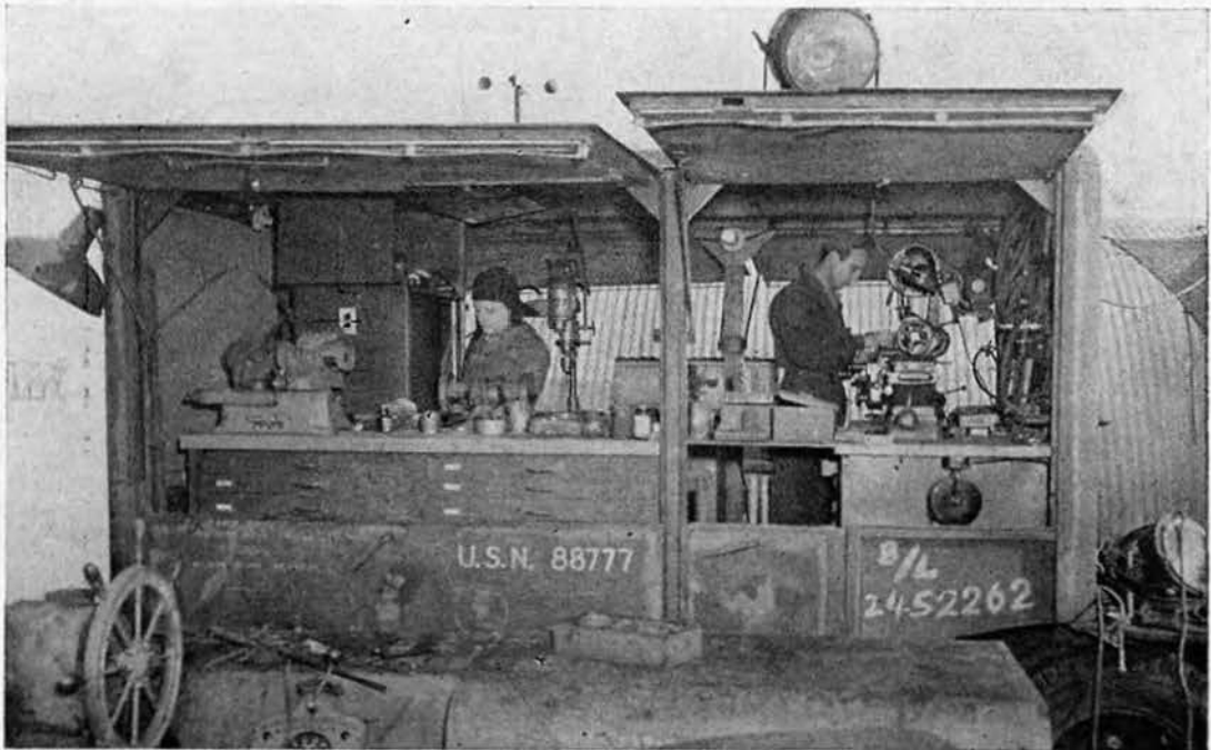
PORTABLE MACHINE SHOP: Installed on repair barge for precision machining operations.
