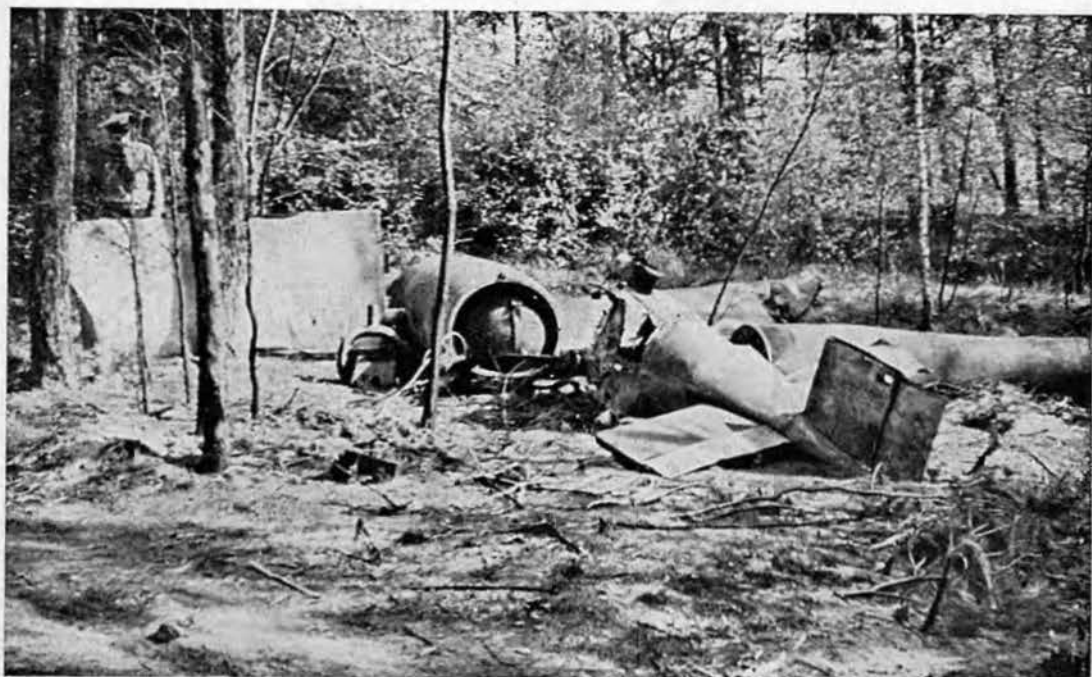
DEFECTIVE V BOMB: Some would plunge to earth a few hundred yards from the catapult. Note the spherical fuel chamber. It is made of rubber wound with steel wire.
