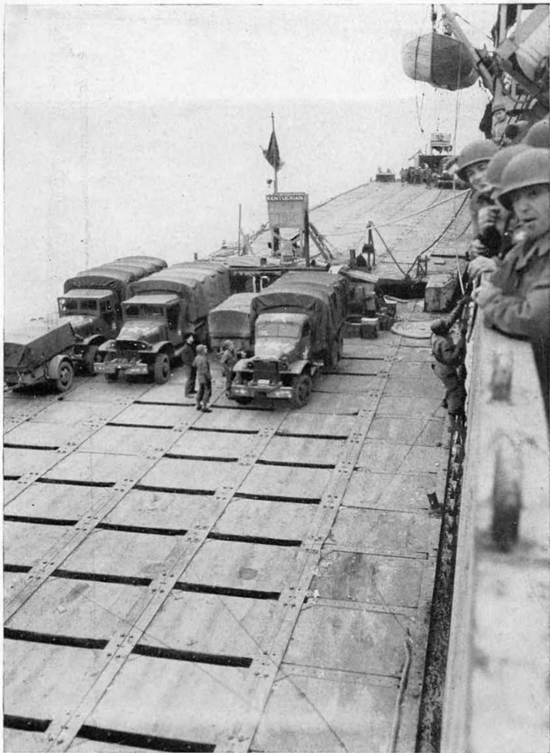
THE RHINO BARGE "KENTUCKIAN" receives its cargo of army trucks from a transport riding at anchor in deep water beyond the Mulberry.
