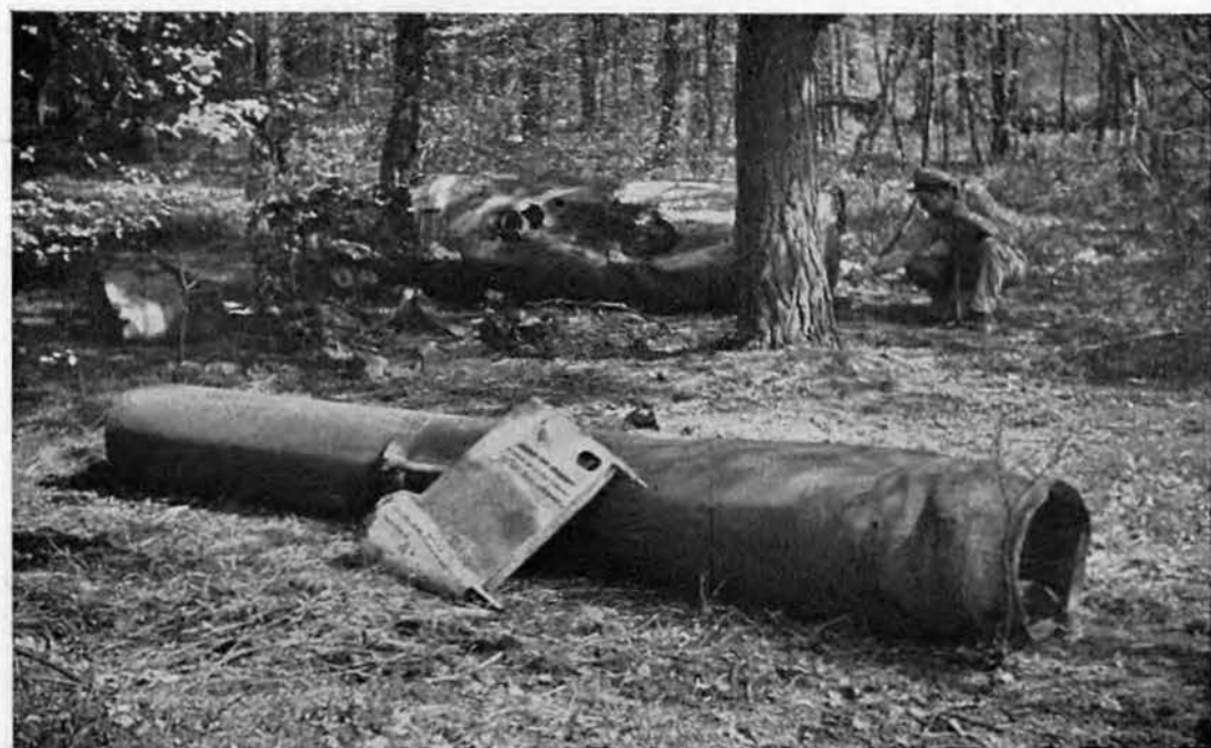
VIEW OF PROPULSION EXHAUST CYLINDER in foreground. Note burnt out war head on section in the background.
