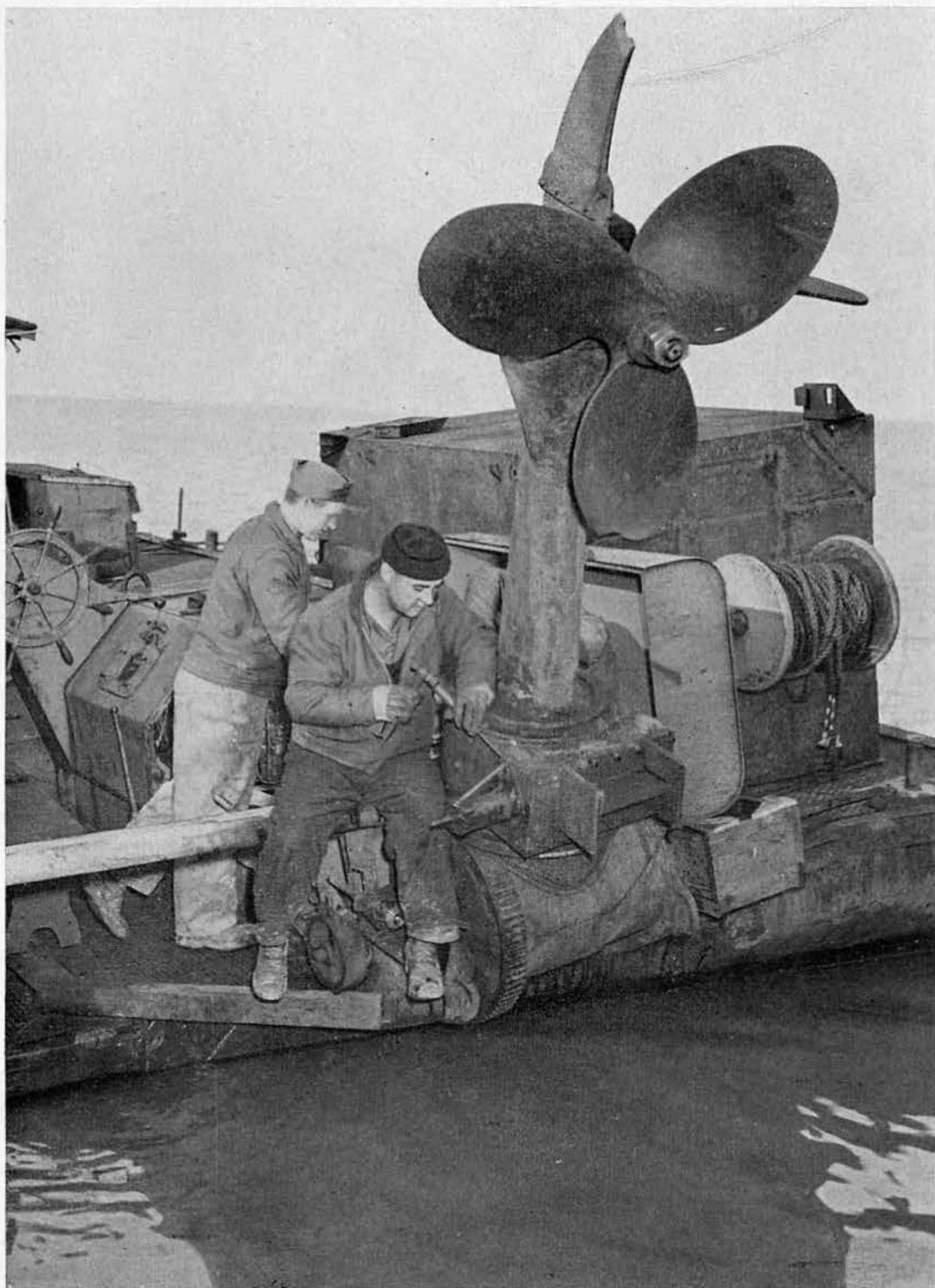
REMOVING PINION GEAR from the housing of a propulsion unit on the repair tug. Underwater obstructions caused damage to the units in shearing off rudder fins and through fouling the screws.
