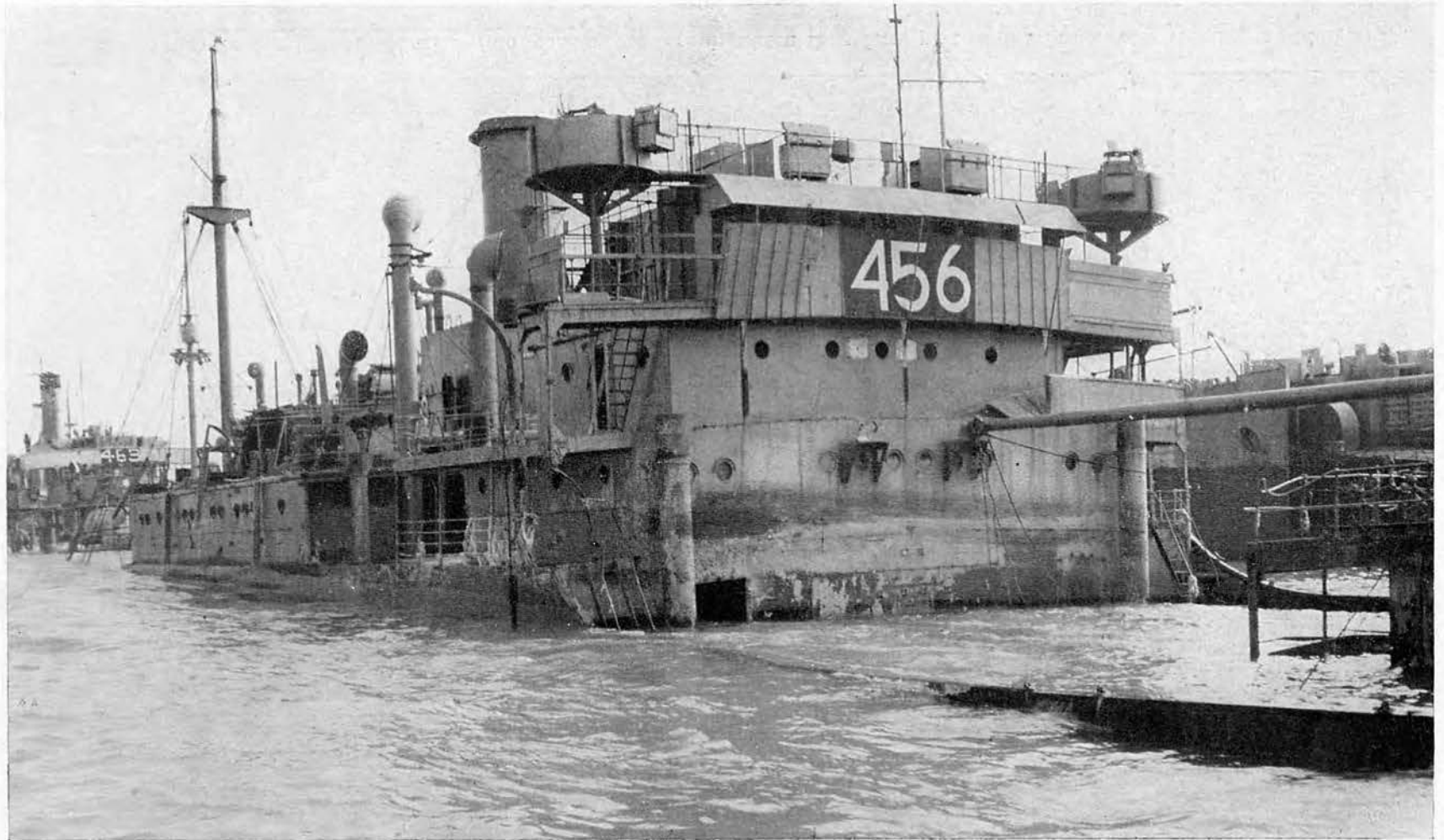
BLOCKSHIPS: Numerous sunken ships extended the breakwater line from the "Phoenixes" parallel along the length of the coast.
