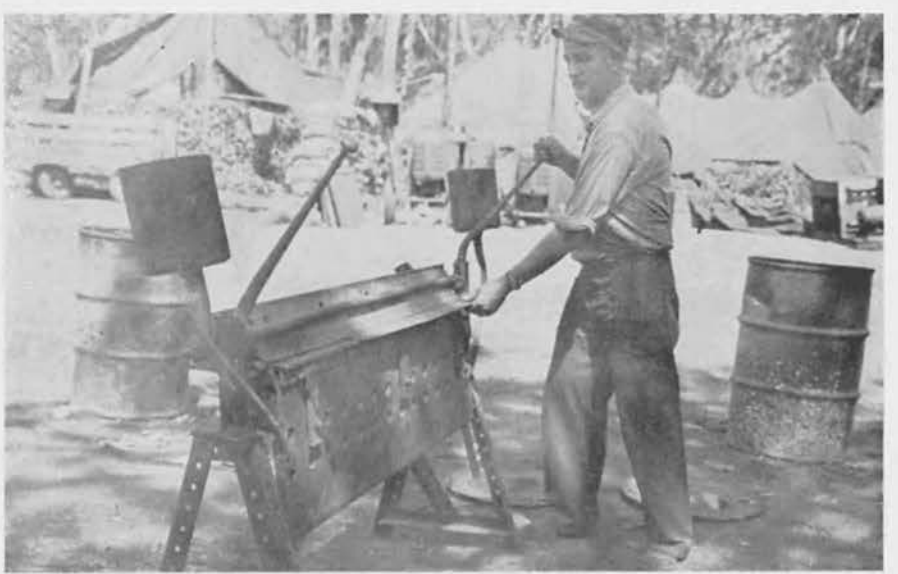
Sheet metal breaker
