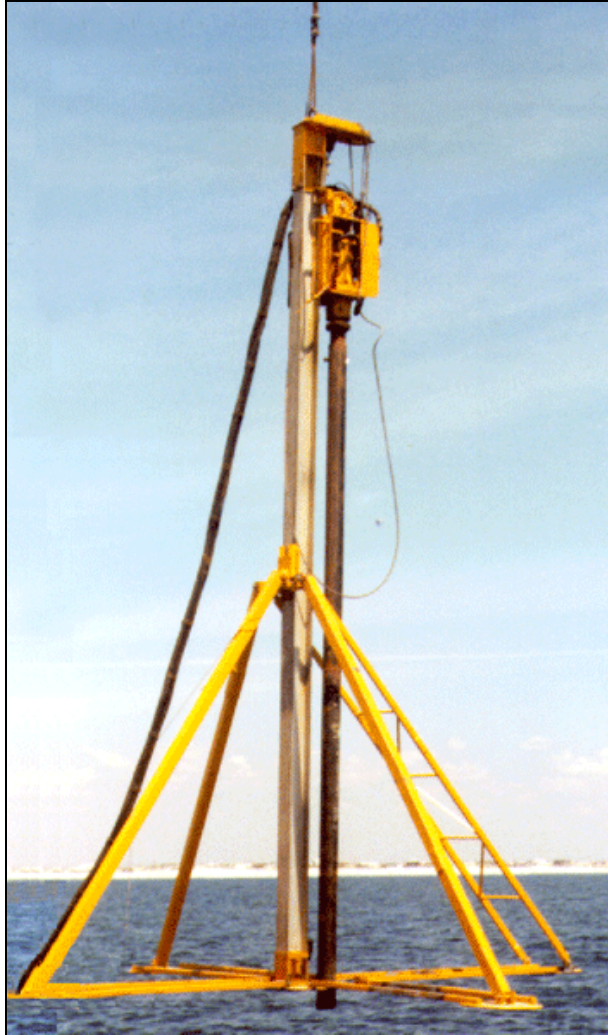
Figure 2.4-4. Alpine vibracore sampler (from Ref. 2-6).
