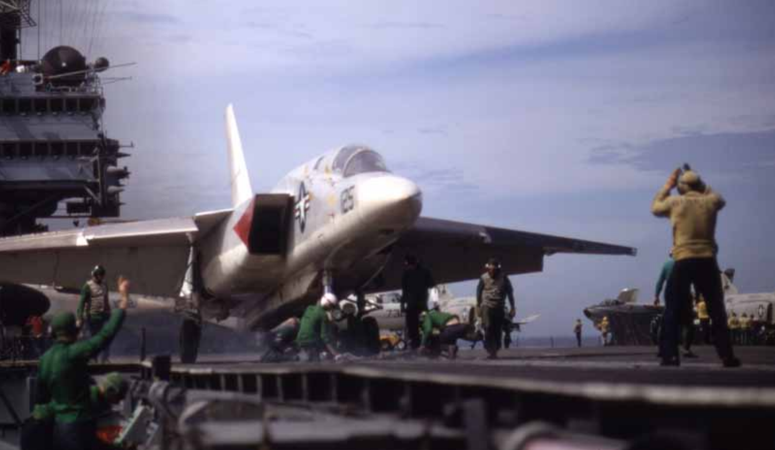
An RA-5C is lined up on the starboard forward catapult of a Kitty Hawk -class carrier. ( National Archives and Records Administration )
