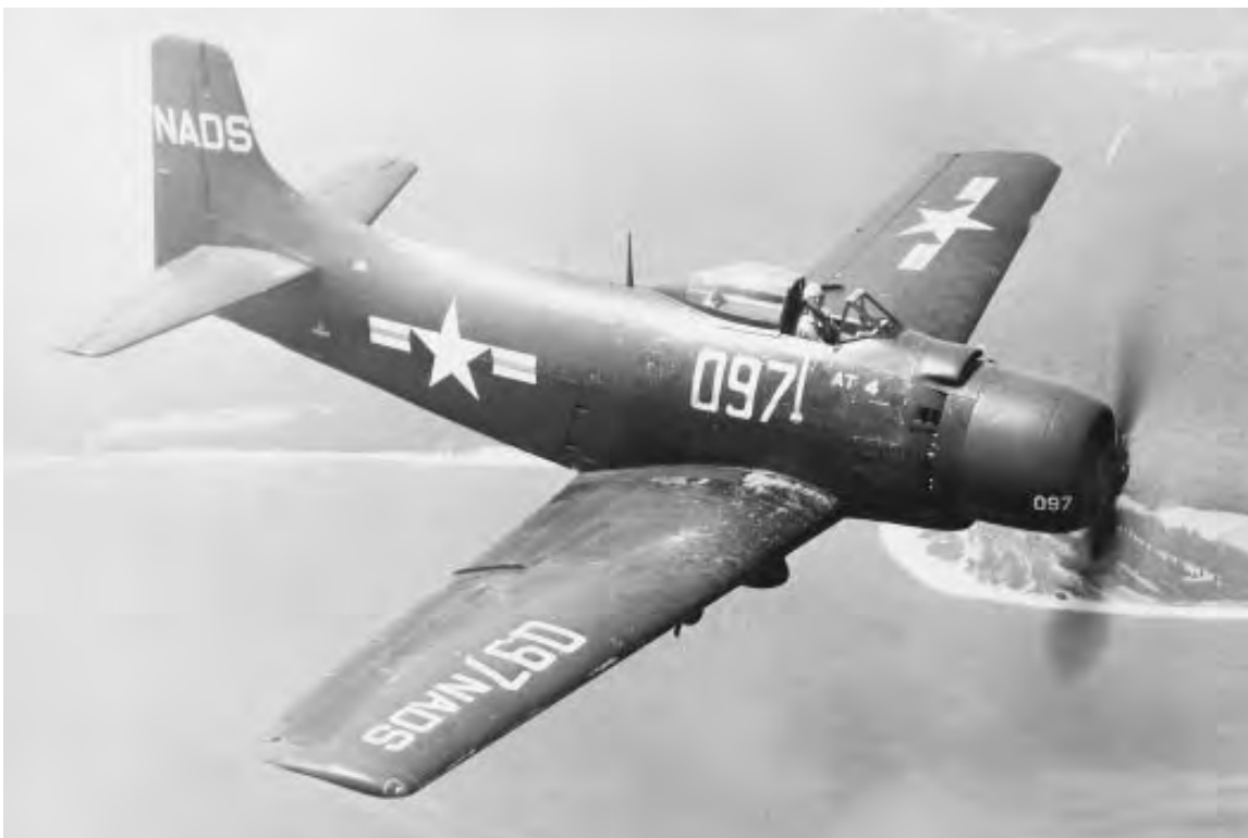
An XBT2D-1 in flight. This was the first designation assigned to the AD Skyraider.
