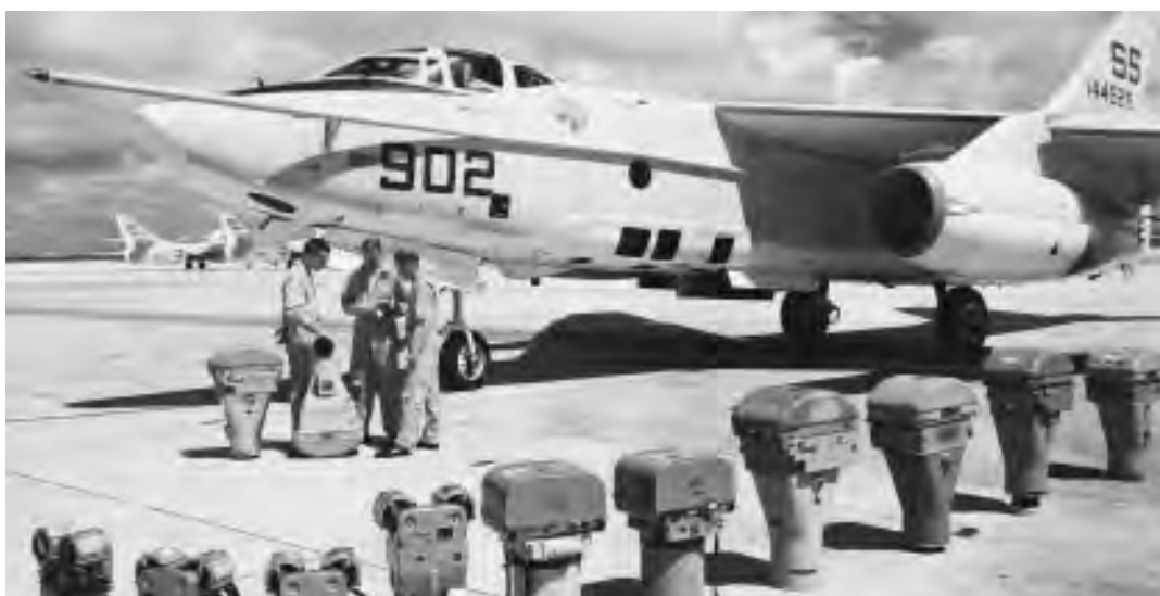
A squadron RA-3B Skywarrior at NAS Agana, Guam, surrounded by a display of aerial cameras used for cartographic and reconnaissance photography taken by the squadron, circa 1965 or 1966.
