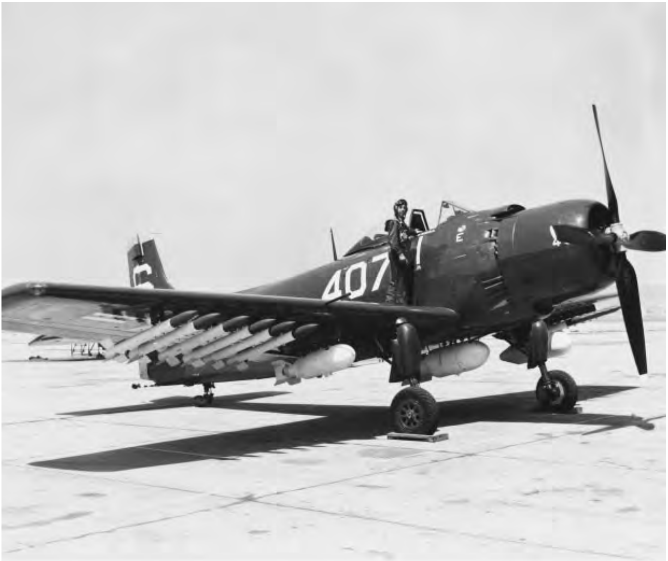
A squadron AD-1 Skywarrior loaded with dud rockets and general purpose bombs. The squadron's joker and card insignia and Battle E award are on the fuselage just forward of the pilot.
