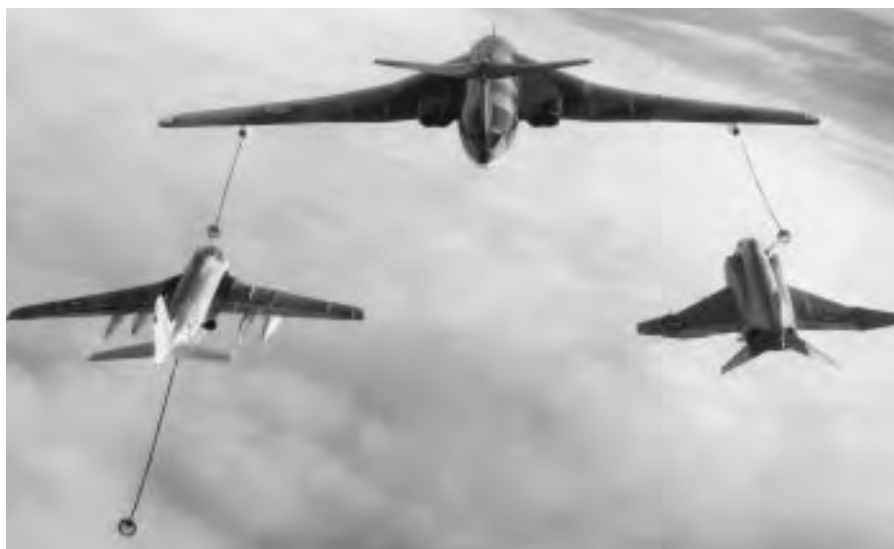
A British Victor tanker refuels a squadron KA-6D Intruder and an F-4 Phantom II. Note the refueling line and basket being trailed by the squadron's KA-6D.
