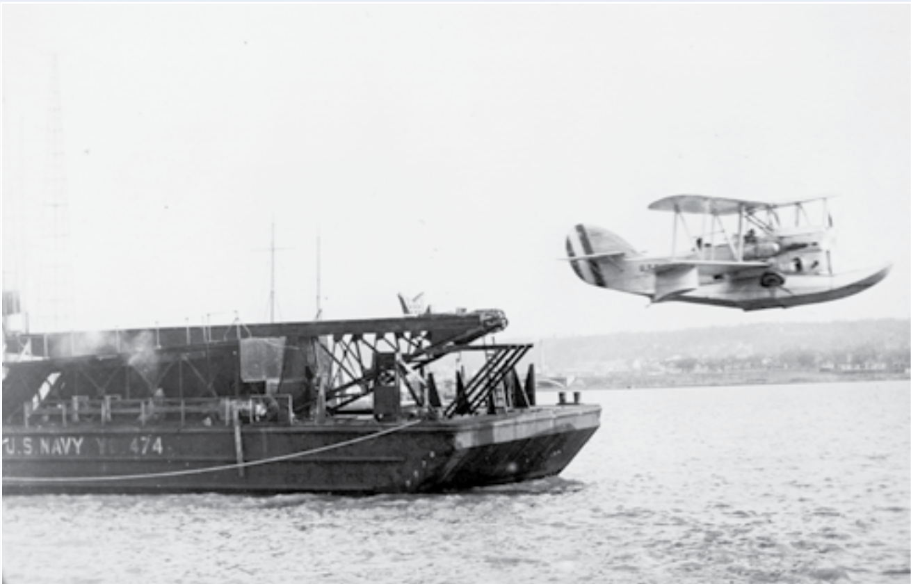
A seaplane is launched by catapult from a navy yard barge operating in the Anacostia River during tests conducted in 1926.
